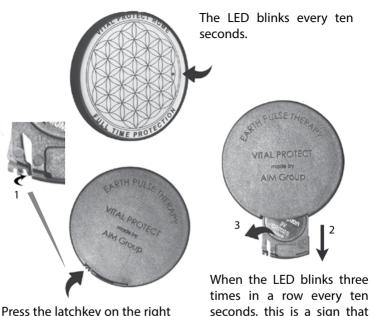
Press the latchkey on the right side and at the same time gently pull out the gliding compartment. When the LED blinks three times in a row every ten seconds, this is a sign that the battery is almost empty. Gently remove and replace it with a new one.
